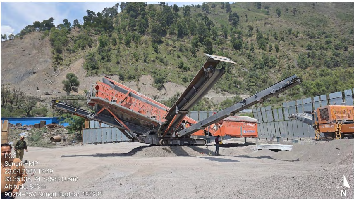
Pic-6: Mobile Stone Crusher
